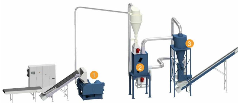
1: Fine Granulator FG1504 2: Zig Zag Separator 3: Cyclone
