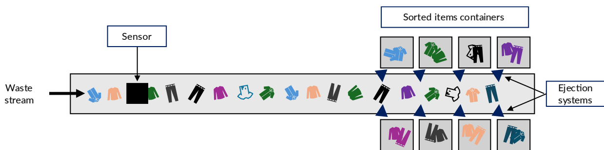
Figure 8: Multi-category sorting line operating diagram
