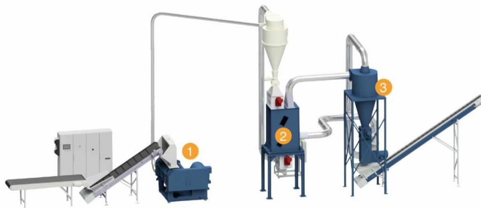
1: Fine Granulator FG1504 2: Zig Zag Separator 3: Cyclone
