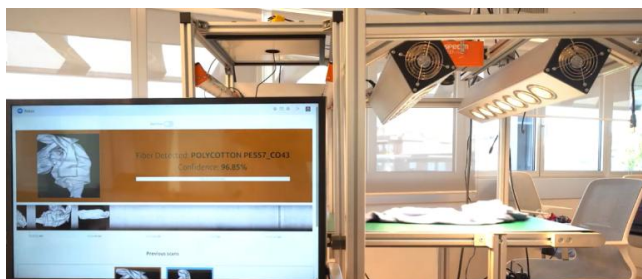
Figure 19 : Specim RETEX test portal
