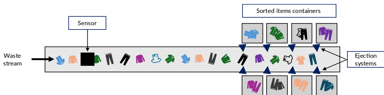
Figure 8: Multi-category sorting line operating diagram
